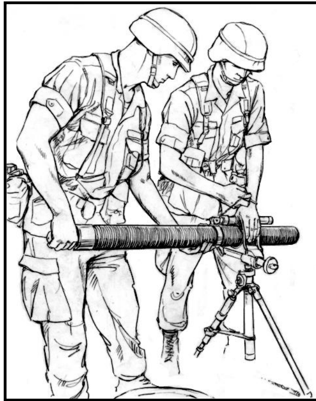
Figure 5-8. Bipod and mount attachment ring secured.
